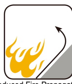
Reduced Fire Propagation NF C32-070-2.2(C1) IEC60332-3-24 EN50266-2-4
